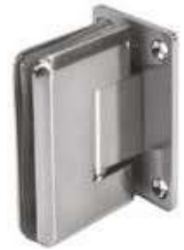
PCA-SH01 Glass - Wall Hinge 10mm | Glass Thickness 40 kg | Max. Weight Zinc Alloy, Stainless Steel 304 | Material Satin, Polished, Black Anodize | Finish
