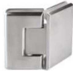
PCA-SH05 135° Glass - Glass Hinge 10mm | Glass Thickness 40 kg | Max. Weight Zinc Alloy, Stainless Steel 304 | Material Satin, Polished, Black Anodize | Finish
