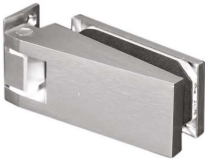
PCA-DH13 Door Hinge 10mm | Glass Thickness 50 kg | Max. Load Aluminium | Material Natural Anodize, Satin, Black | Finish
