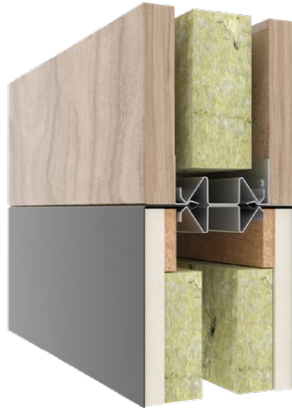
Seamless connection with 0 joint between panels with different finishes.
